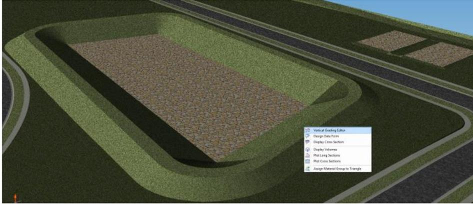
The grading tools support cross section templates and intelligent daylighting/batters to address any site design requirements. The surface and grading linework automatically updates as you edit your grading, so you get dynamic feedback on the impact of your design changes. Get volume outputs at the click of a button.
